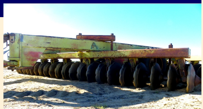
Above: A offset disk plough used for lime incorporation at Wubin
