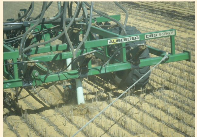
Above: DBS unit sowing on 500mm rows at 5kph, note less soil throw to cover inter-row.
