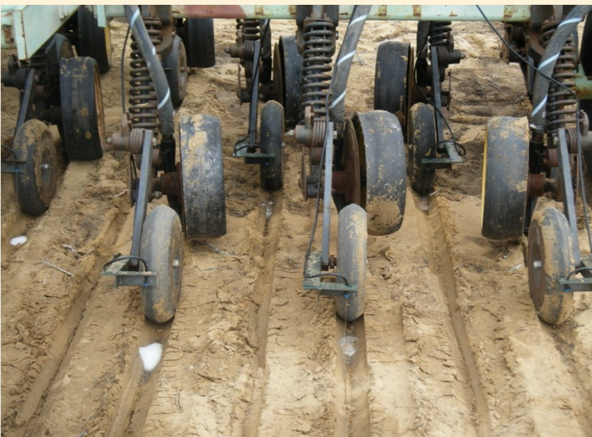
Above: Banded surfactant behind presswheels of a Germinator single disc bar with depth control wheels.
