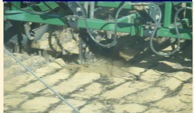
Above: DBS unit sowing on 500mm rows at 10kph, note soil throw to cover inter-row.
