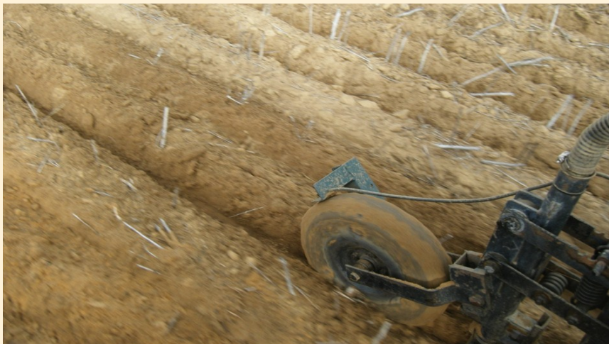
Above: This V press wheel throws less soil than the rectangular presswheel below and is therefore more suited to use with banded wetting agents.
