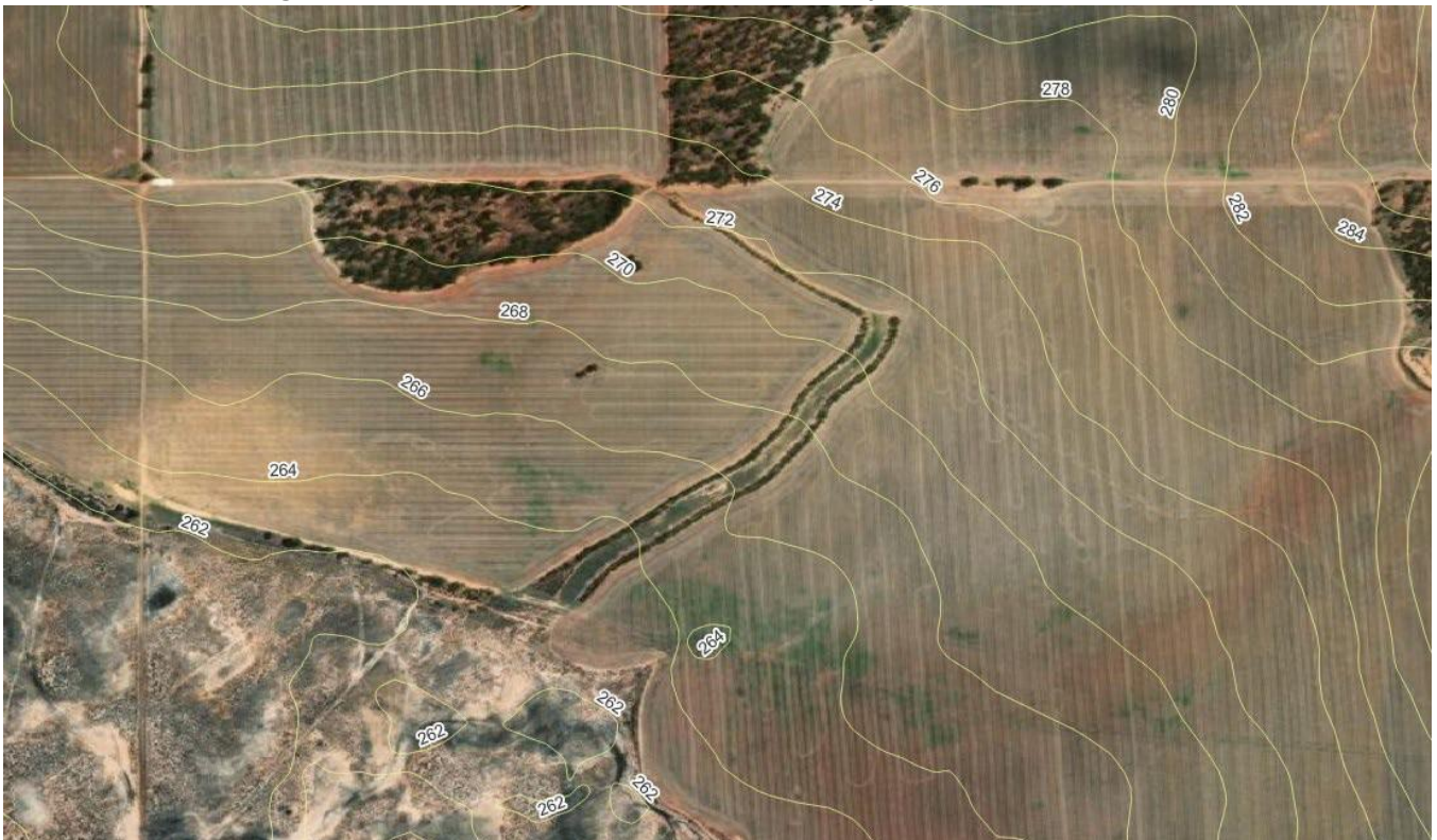
Figure 7.3 Grade bank and grassed waterway in the project catchment
